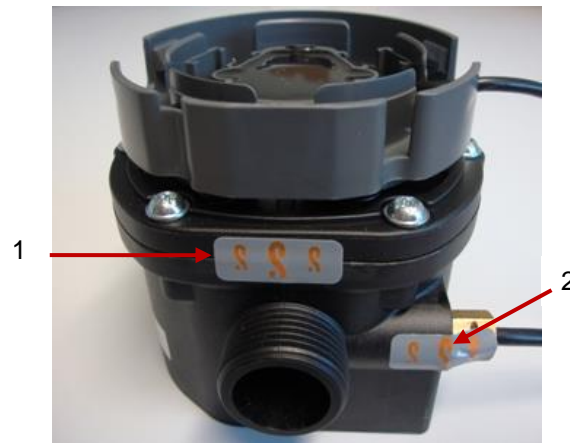
Seals installed in the factory on flow meter (1) and temperature sensor (2) of the Superstatic 789
